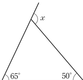
$$\begin{aligned} \angle x &= 65^\circ + 50^\circ \\ &= 115^\circ \end{aligned}$$
